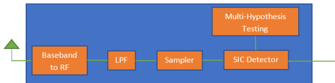
Fig. 3. A generic receiver model for the proposed MAC protocol
